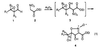
This reaction can be depicted as a base-catalyzed tandem nitroaldol cyclization process in which the chainlengthening step affords a 2-nitroalkanol 3 and/or its aci-nitro form as transient species that undergoes a fast epoxide ring-opening cyclization to 4.
